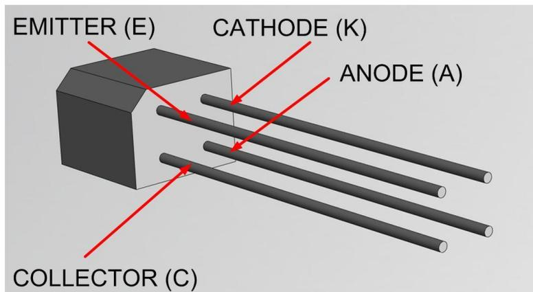
Identify the leads from the diagram and connect to the terminals marked A, K, C and E on the PCB.
