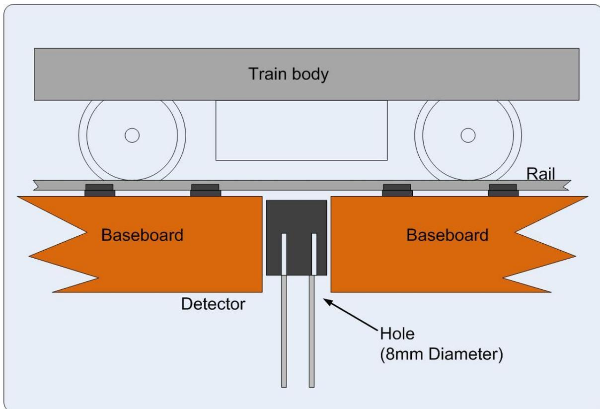
The detector can be mounted in an 8mm hole drilled through the track baseboard. If required, the detector can be held in place using a small amount of blutack, expanded polystyrene or similar.
