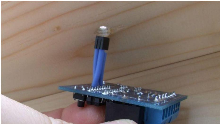
The module detects trains by bouncing invisible Infra-Red (IR) light off the underside of the rolling stock, and detecting the light reflected back. The modules are fitted to the underside of the baseboard, and the sensor sits level with the track bed.
