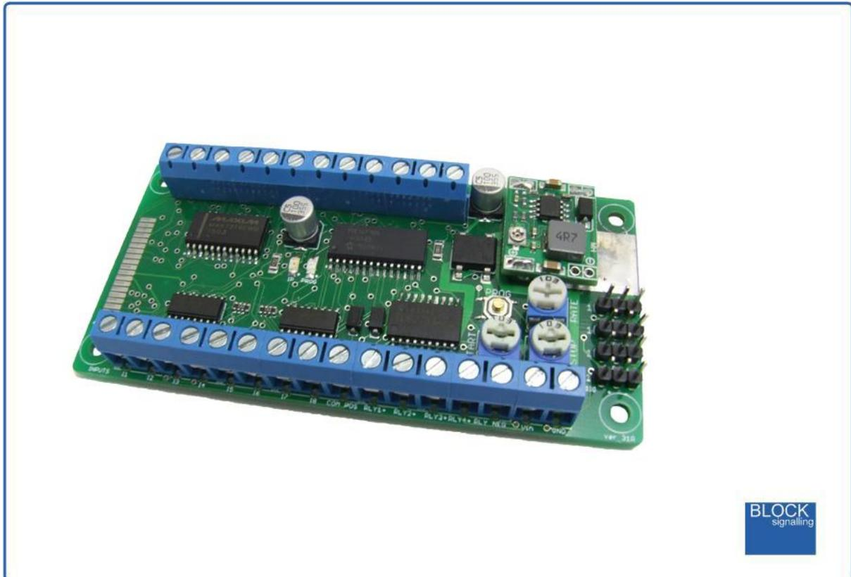
The BLOCKsignalling Smart ServoSwitch SRV4 is designed to operate up to four servos between their Start and Stop positions, whenever a control input is switched.
