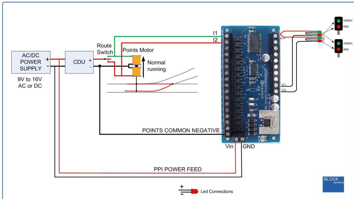
Here is a close-up of the wiring necessary.
