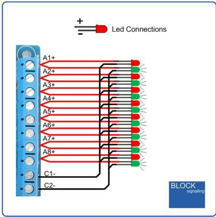
Following factory testing, sometimes more than one led will be lit. This will clear as soon as each set of points is first operated.
