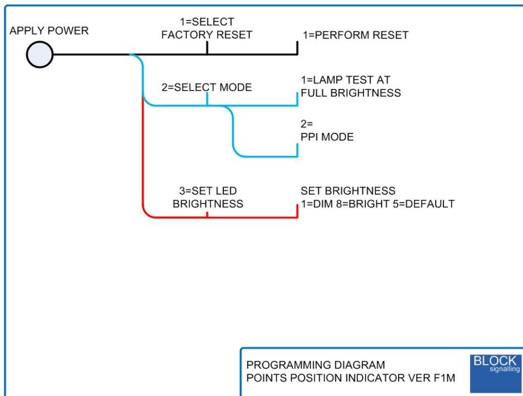
If the button is pressed whilst the PPI is running, it will perform a led test sequence.
