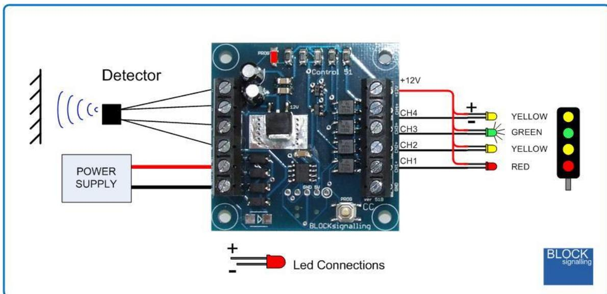
This program simulates the operation of a four aspect signal, which is normally showing green. The module searches for a train, and if one is detected in front of the sensor, the signal immediately switches to red.
