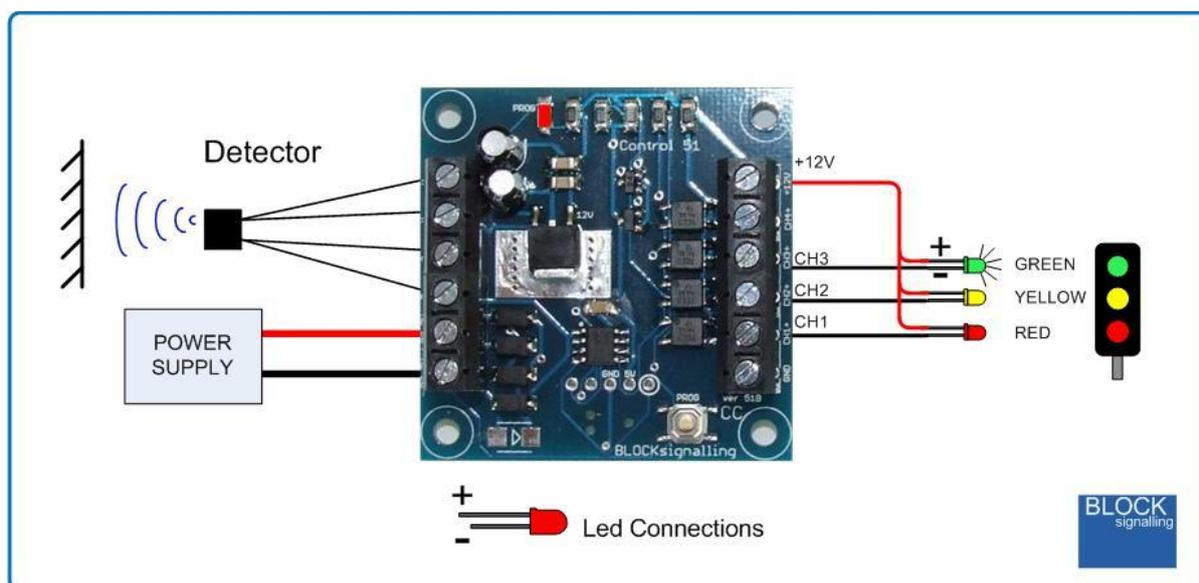
This program simulates the operation of a three aspect signal, which is normally showing green. The module searches for a train, and if one is detected in front of the sensor, the signal immediately switches to red.
