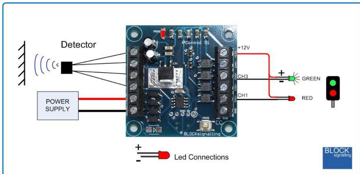
This program simulates the operation of a two aspect signal, which is normally showing green. The module searches for a train, and if one is detected in front of the sensor, the signal immediately switches to red.
