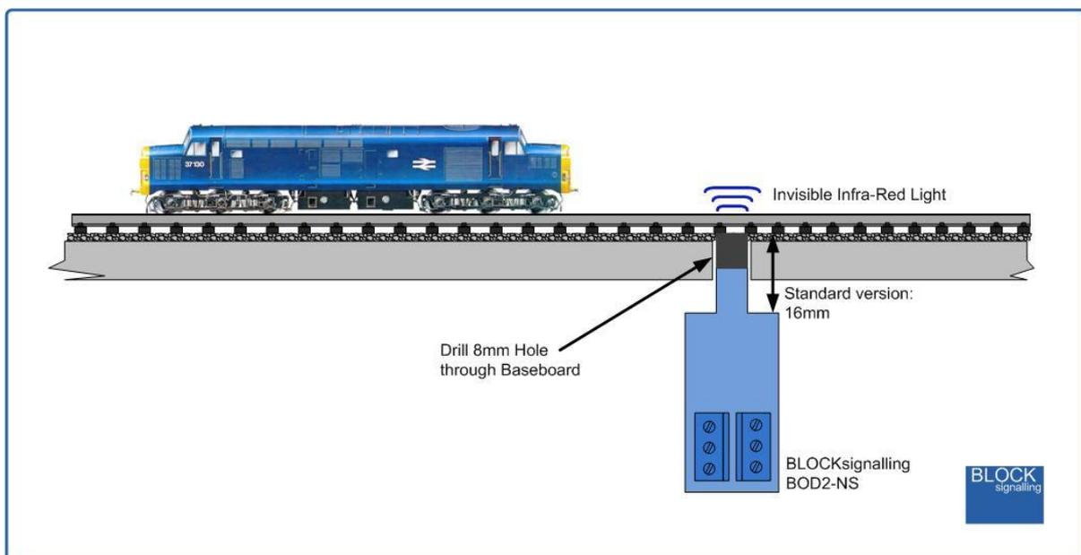
If required, the sensor can be held in place using a small amount of blutack, expanded polystyrene or similar.
