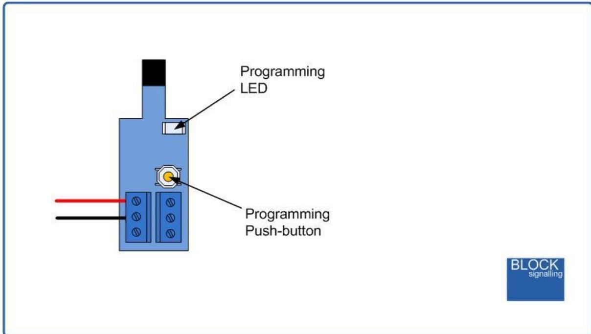
The red led on the PCB flashes at 1 second intervals. When the required number of flashes is seen (see later for the list of possible choices) the button is released to store the first value. At this point the led comes on for five seconds to confirm the value is stored.
