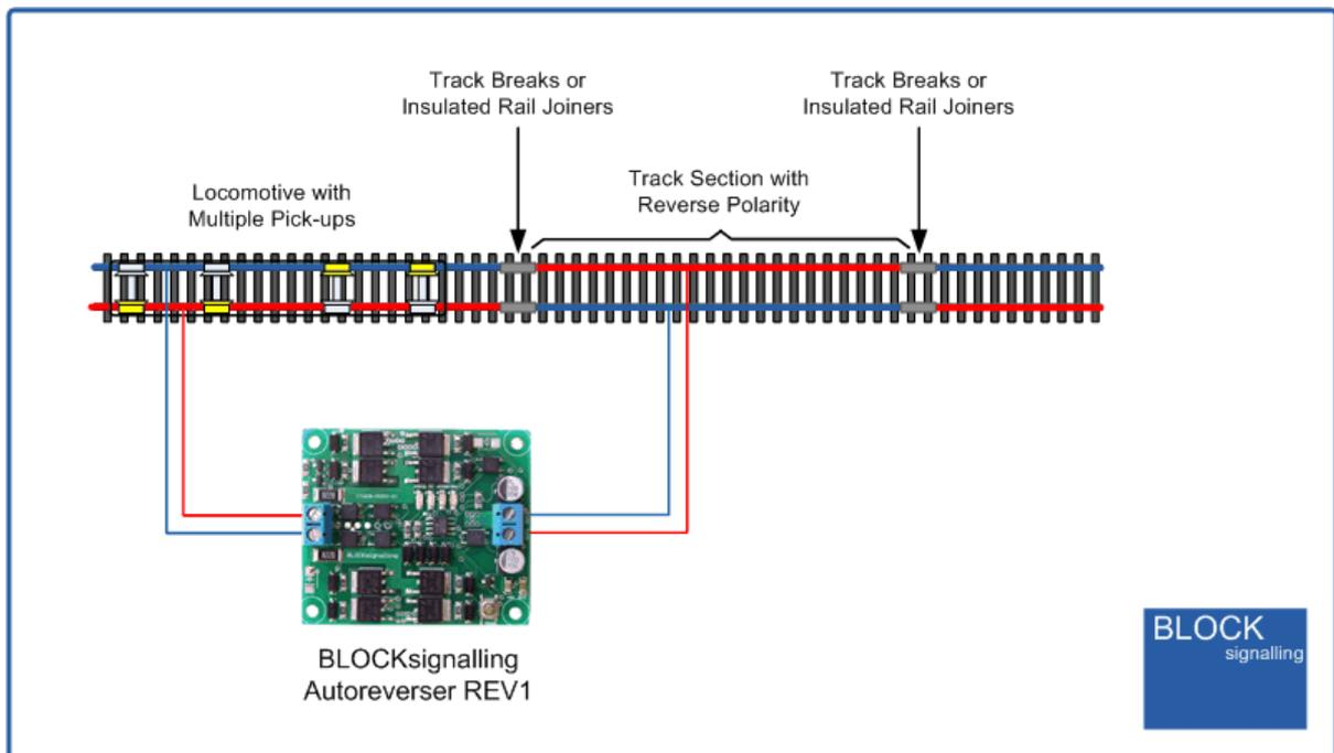
As the train moves to the right, it crosses the rail breaks and enters the central section of track.
