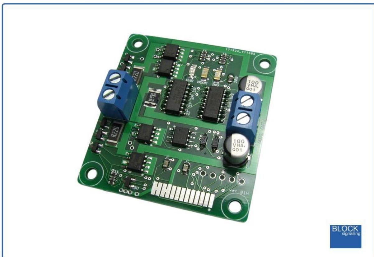
Autoreversers are used on DCC layouts to automatically switch the polarity of track feeds in layout features such as loops, wyes and to provide feeds for turntables.
