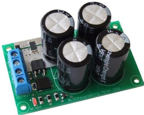
The BLOCKsignalling CDU4R has a red LED on the PCB that lights when the capacitors are charged to 15V and above. Knowing the state of the charge on the capacitors is useful to confirm correct supply connection and to show that the capacitors are charged sufficiently. The led will also indicate if a points switch has inadvertently been left operated, as the LED will not re-light after the points operation.
