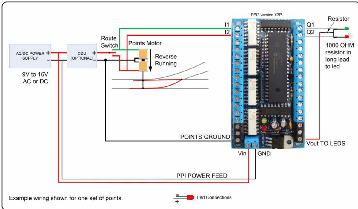
System Operation – with separate power supplies for points and PPI.
