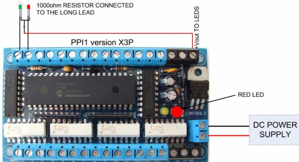
1. CONNECT DC POWER SUPPLY (BETWEEN 8V AND 16V)
