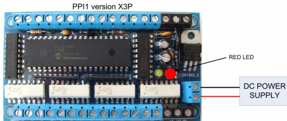
1. CONNECT DC POWER SUPPLY (BETWEEN 8V AND 16V)
