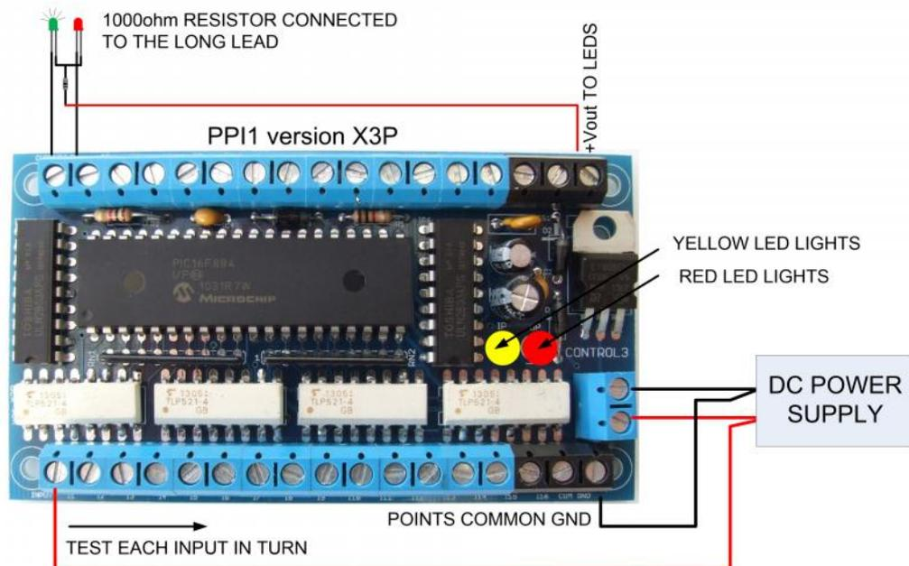
1. CONNECT UP POWER SUPPLY AND LEDS ON THE OUTPUT AS IN TEST 3
