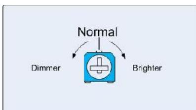
Operating the leds at the minimum acceptable brightness level will prolong the life of the leds.
